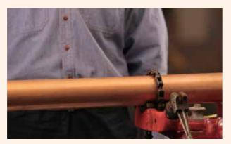
**5.** Secure the tube in a vise or pipe support to prevent any movement of the tube and insert the fitting onto the tube. Ensure the outer edge of the fitting lines up with the insertion depth mark made in step 4.
