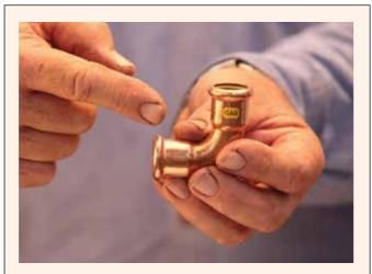
**6.** Ensure you have the correct fitting for the application (e.g. water or gas). Check the fitting is clean and the O-ring is free from debris and correctly sitting in place. Push fitting on tube all the way to the engagement marking.
