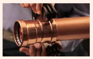
**7.** Open the collar and place it around the fitting, such that the bump on the fitting is rested into the groove of the pressing collar. Close the press collar ensuring it fits square with the fitting and check the insertion depth mark still lines up with the outer edge of the fitting.
